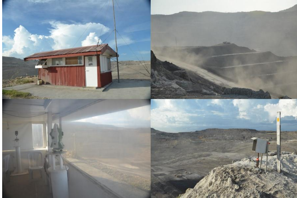
Figure 13. The GEOMOS. From top left, clockwise: the total station located at the east wall of Panian Expansion Pit; a view of the total station from a prism station (lower right picture); the Leica Viva TS15 inside the total station. (Source: GPPamintuan)
